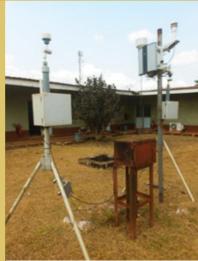
Air quality monitoring station (OIZOM Polludrone)
